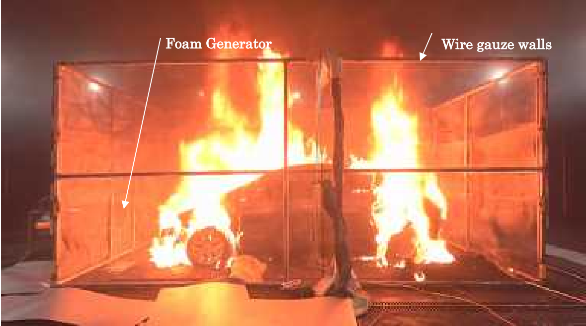
Figure 2: Test vehicle on intensified fire
